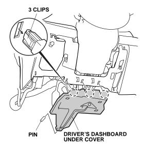
6. Gently pull out the center console, and remove the one clip. Remove the driver's center lower cover (one clip and two hooks).
