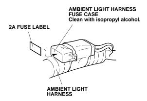
12. Plug the ambient light harness 5-pin connector to the vehicle stability assist 5-pin connector unplugged in step 4.
