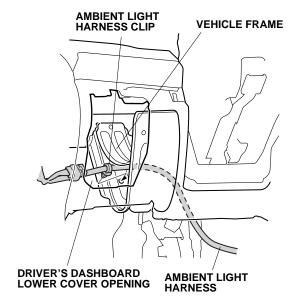
15. Attach the remaining ambient light harness clip to the tab on the dashboard frame.
