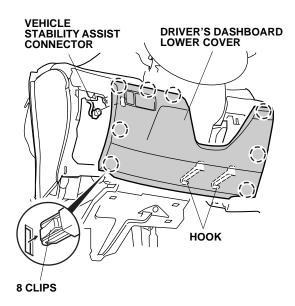
5. Remove the driver's dashboard under cover (three clips and one pin).
