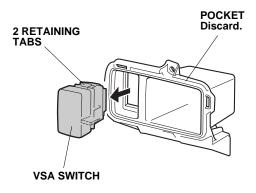
9. Install the VSA switch (removed in step 8), and the ambient light switch into the switch trim.
