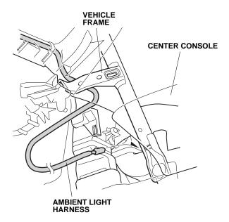
18. Route the ambient light harness through the center console towards the passenger's side of the vehicle. Using one wire tie, secure the ambient light harness to the vehicle frame.
