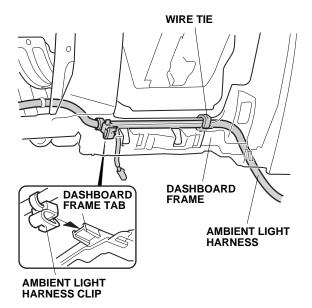
16. Using one wire tie, secure the ambient light harness to the dashboard frame.
